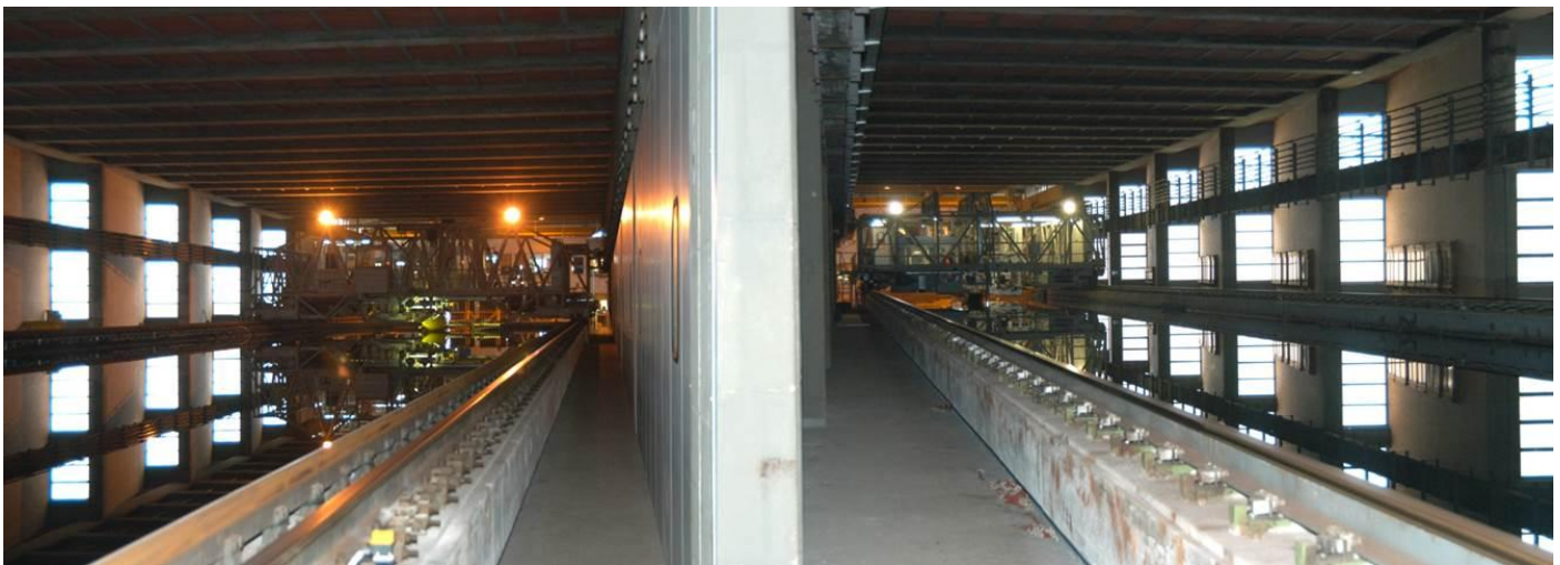
Figure 2: Wave (left) and calm water (right) towing tanks at CNR INSEAN.
